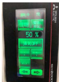
Low air volume (push/pull type), ultrahigh speed variable air volume (VAV) local ventilation device (exhaust fan output visualized on the operation panel) (Minase Research Institute)
